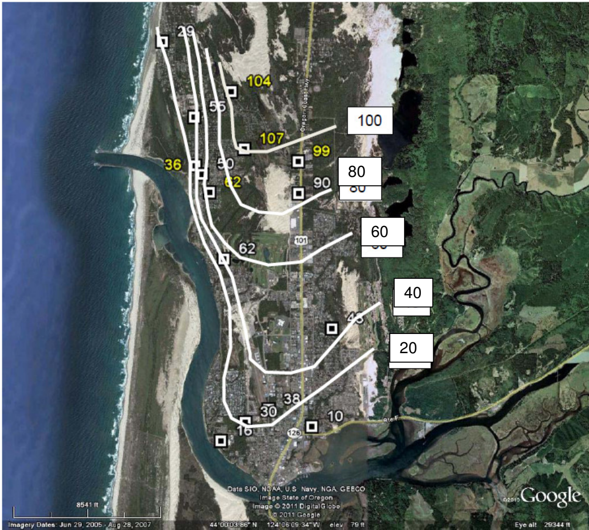
Figure 2. Approximate water table elevations in the Florence area. White numbers represent measurements in early March, 2011; yellow numbers represent data from new monitoring wells installed at the end of March, 2011. Water table contour elevations are feet above mean sea level. Groundwater gradient is much steeper to the west than to the south.
